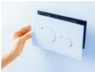
To remove the push plate, simply grasp behind the plate, then pull and swivel the plate downwards.
