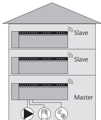
**Note:** The base station the components are connected to must be configured as master. Further base stations can only be paired with the master.
