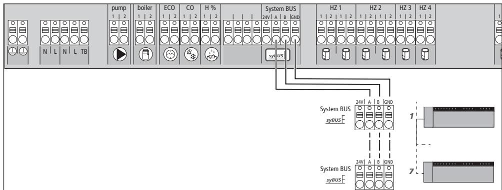
A maximum of seven base stations can be interconnected via the system BUS (syBUS) in order to exchange global system parameters. After completing the wiring, the base stations must be paired – see section 4.2. For a line diameter <6 mm, a strain relief must be provided by the customer.
