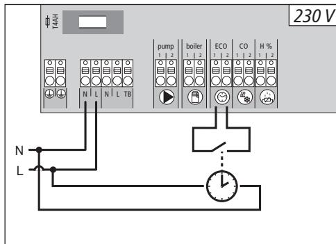
The base station is equipped with an ECO input for connecting an external timer, if the internal clock of the room control unit Radio Display shall not be used. When the input is activated by the timer, the heating zones are switched to night operation.
