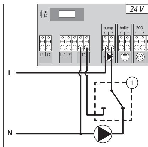
Connection of a customer-supplied temperature limiter (1). This device switches off the pump and sets the input to TL if too high flow temperatures for the floor heating are detected. If the TL input is switched, the base station shuts down all actuators automatically.
