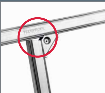
Inaccuracies (of up to 10 mm) when cutting the section tube to length can be easily rectified by the corner joint.
