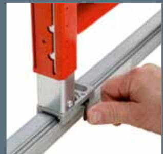
After the module feet have been locked, the module is permanently connected with the lower continuous profile brace.
