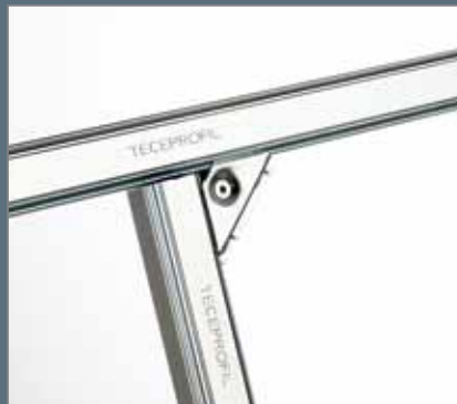
The beading in the edge area of the section tube holds the corner joint tightly and also improves the tube stability.
