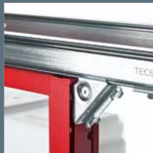
The slotted profiles in the module frame enable the modules to be fixed to the supporting framework with corner joints.
