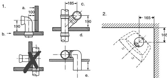
**1. S+Q a.** Finished wall **b.** Finished floor **c.** Drainage pipe dim 110/45 **d.** WC-connection **e.** Cut to suitable length
