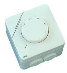
THYRISTOR CONTROLLER VRS. For manual variable speed control of single-phase motors. Minimum speed is adjusted by means of a screw under the knob. The controller is certified and approved as conforming to electrical safety and interference regulations on all markets. All single-phase fans from Östberg can be regulated with VRS controller.
