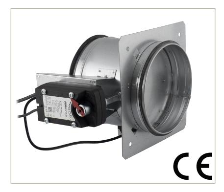
Fire and smoke damper ETPR-E-1 is used as a closing device for preventing the spread of fire and smoke in ventilation ducts between fire compartments. Fire dampers are equipped with fusible link and spring mechanism for closing or with electrical actuator.
