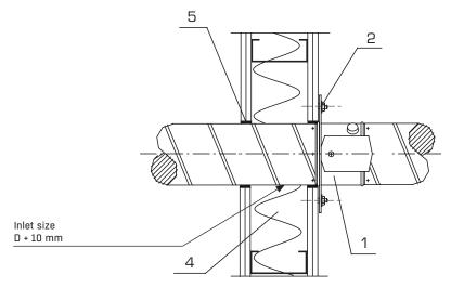
Installation of fire damper into lightweight plasterboard building elements (gypsum board or similar), wall thickness  $\geq$  116 mm. The blade shaft can be placed in any position.
