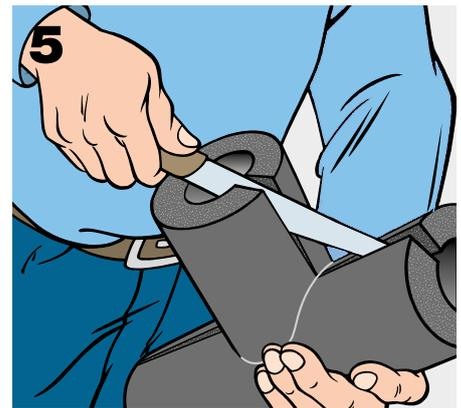
Stick the insulation to the T-junction. Then the three straight tube sections can be attached and glued together.
