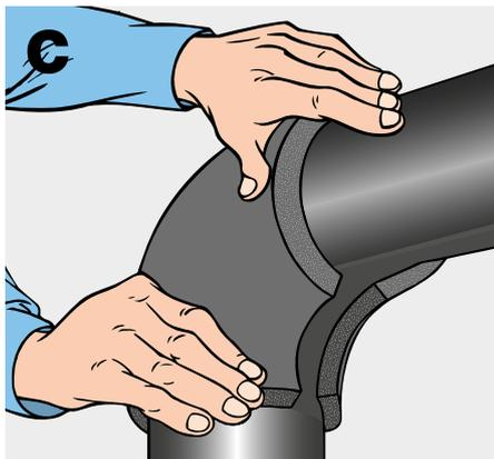
Bond the glued edges together by applying pressure.
