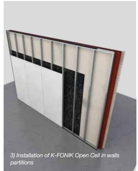
**3) Installation of K-FONIK OPEN CELL in walls partitions**
